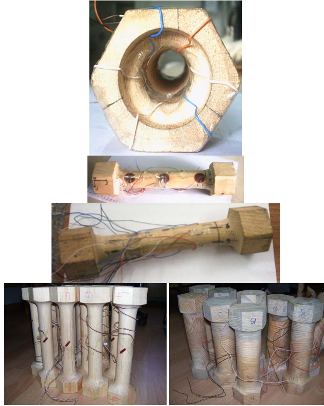
Figure 6. Pinewood specimens with strain gauges.
