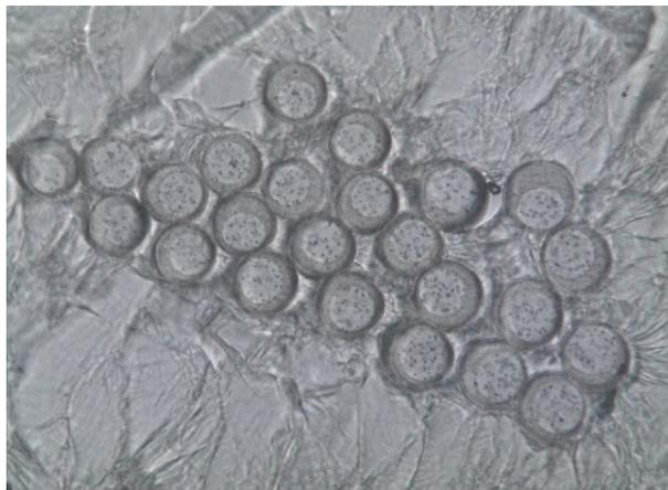
**Figure 1.** SEM of S/C type of developed FR yarn (S: nano-TiO<sub>2</sub>, C: FR PET/original magnification 400×).
