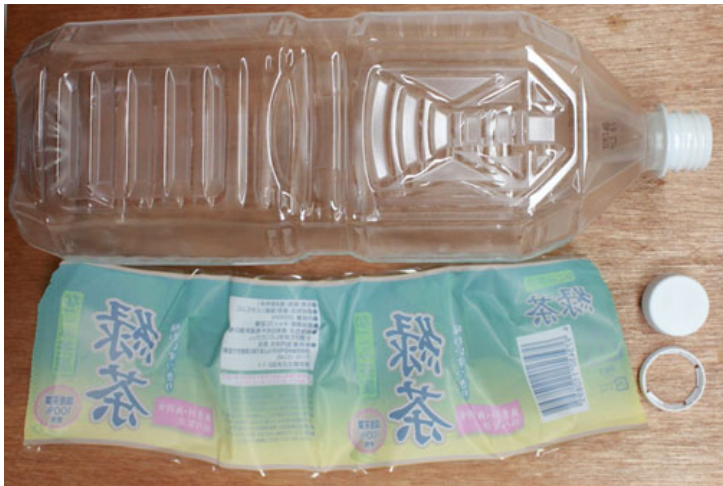
Figure 1. Photograph of waste PET bottle, PE or PP cap, and PS label.
