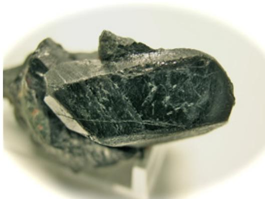
**Figure 1.** Ilmenite ore. Picture obtained from virtual museum of the University of Huelva.
