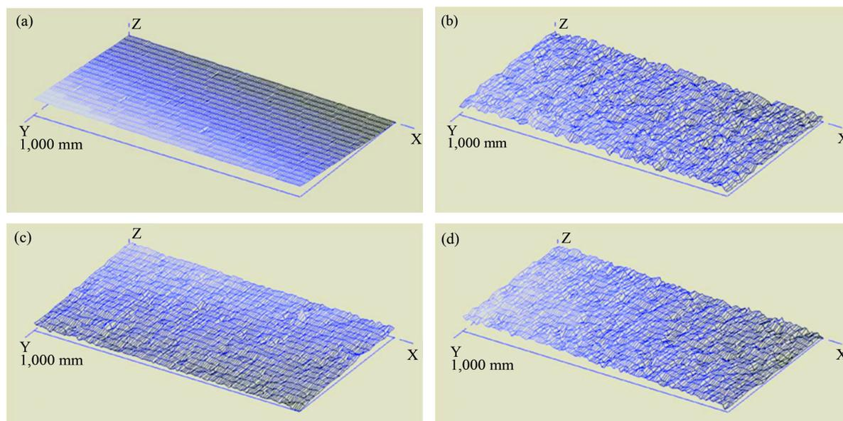
**Figure 3.** Computer generated topography images of the (a) Polished, (b) Sandblasted, (c) Sandblasted &  $\text{TiO}_2$  coated, (d) Sandblasted & acid etched surfaces.
