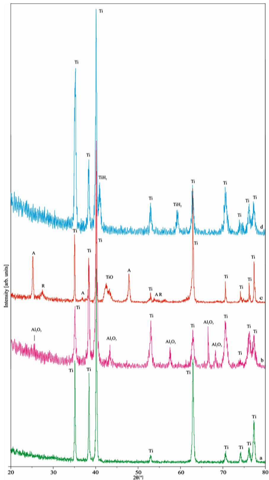
**Figure 5.** XRD patterns of (a) Polished, (b) Sandblasted, (c) Sandblasted &  $TiO_2$  coated, (d) Sandblasted & acid etched surfaces. A: Anatase, R: Rutile.
