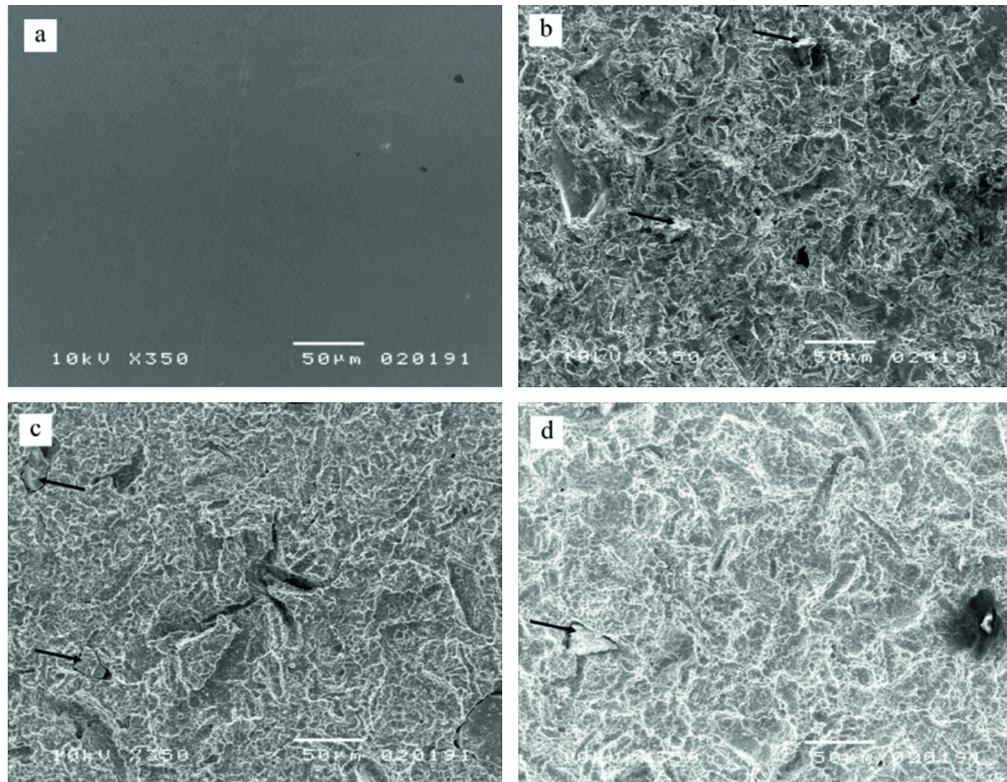
**Figure 4.** Scanning electron micrographs of the (a) Polished surface, (b) Sandblasted surface, embedded  $\text{Al}_2\text{O}_3$  particles (arrow), (c) Sandblasted &  $\text{TiO}_2$  coated surface, embedded  $\text{Al}_2\text{O}_3$  particles coated with  $\text{TiO}_2$  (arrow), (d) Sandblasted & acid etched surface, embedded  $\text{Al}_2\text{O}_3$  particles (arrow) (original magnification  $\times 350$  and bar =  $50\ \mu\text{m}$  except where stated).
