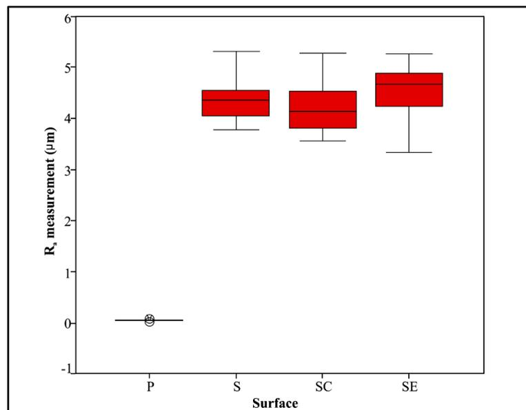
**Figure 1.**  $R_a$  (average roughness) surface roughness assessment of the Polished (P), Sandblasted (S), Sandblasted &  $\text{TiO}_2$  coated (SC), and Sandblasted & acid etched (SE) surfaces. Data are reported as mean  $\pm$  SD.
