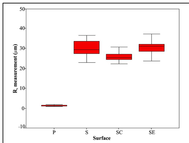
**Figure 2.**  $R_z$  (mean roughness depth) surface roughness assessment of the Polished (P), Sandblasted (S), Sandblasted &  $\text{TiO}_2$  coated (SC), and Sandblasted & acid etched (SE) surfaces. Data are reported as mean  $\pm$  SD.
