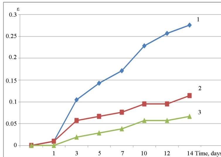
Figure 2. Expansion  $\varepsilon$  (%) of samples with the addition of  $\text{Al}(\text{OH})_3$  "SiTau" stored in 1 M NaOH versus time (days): 1—0% of  $\text{Al}(\text{OH})_3$  (by weight of cement), 2—1%, 3—3%.
