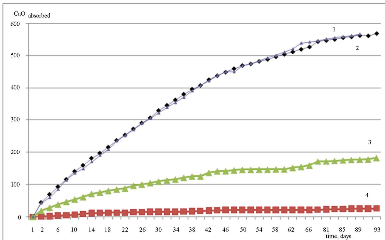
**Figure 1.** The absorption of CaO (mg/g) by aluminum hydroxides versus time (days): 1—SiTau, 2—Geloxal, 3—GD18 (additionally grinded), 4—GD18.
