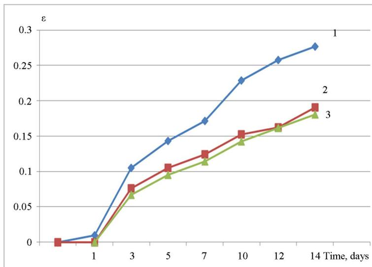
Figure 5. Expansion  $\varepsilon$  (%) of samples with  $\text{Al}(\text{OH})_3$  “GD18” (after additional grinding) stored in 1 M NaOH versus time (days): 1—0% of  $\text{Al}(\text{OH})_3$  (by weight of cement), 2—1%, 3—3%.
