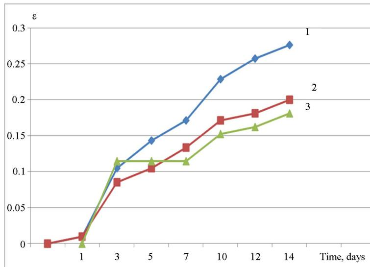
Figure 4. Expansion  $\varepsilon$  (%) of samples with the addition of  $\text{Al}(\text{OH})_3$  “GD18” stored in 1 M NaOH versus time (days): 1—0% of  $\text{Al}(\text{OH})_3$  (by weight of cement), 2—1%, 3—3%.
