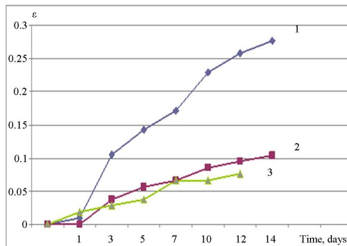
Figure 3. Expansion  $\varepsilon$  (%) of samples with the addition of  $\text{Al}(\text{OH})_3$  "Geloxal" stored in 1 M NaOH versus time (days): 1—0% of  $\text{Al}(\text{OH})_3$  (by weight of cement), 2—1%, 3—3%.
