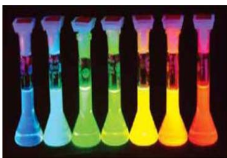
Figure 5. Fluorescence in different-sized CdSe QDs [12].
