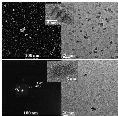
**Figure 3.** SEM, HRTEM and TEM images of Ag<sub>2</sub>S nanoparticles prepared from Ag(I)-Cyanex® 471 solutions at two different ligand concentrations (Ag<sup>+</sup> 0.005 mol/L, upper figure: Cyanex® 471x 0.01 mol/L, down: Cyanex® 471x 0.05 mol/L).
