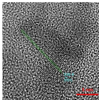
Figure 6. Illustration of lattice image from Ag<sub>2</sub>S nanometric particles.
