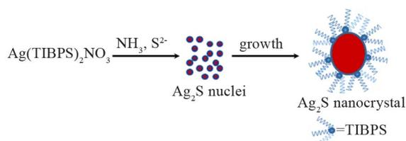
**Scheme 1.** Synthesis of  $Ag_2S$  nanocrystals from silver(I)-loaded Cyanex<sup>®</sup> 471x solutions.
