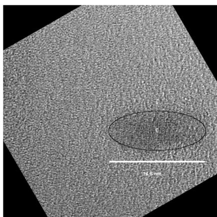
Figure 5. (a) Adjustment to an elliptical shape of the area, and (b) TEM image of Ag<sub>2</sub>S nanoparticle fitting the elliptical shape.
