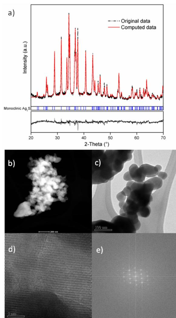
**Figure 2.** (a) Plot of the measured and calculated diffractogram along with the Bragg positions of silver sulphide; (b) STEM; (c) and (d) TEM images and (e) FFT pattern of Ag<sub>2</sub>S from Cyanex<sup>®</sup> 471x solution.
