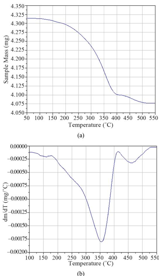
**Figure 8.** (a) Thermal analysis, and (b) maximum rate of mass losses ( $dm/dt$ ) of silver sulphide synthesized from Cyanex<sup>®</sup> 471x solution (0.005 mol/L), 0.01 M  $Ag^+$  in  $HNO_3$  0.1 mol/L.
