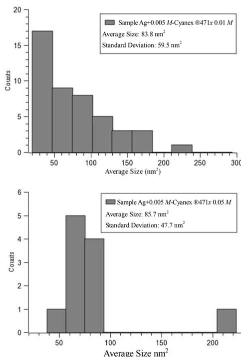
**Figure 4.** Histograms of the particle size distribution as determined from TEM images for the two Ag<sub>2</sub>S nanocrystals samples. A1: Ag<sup>+</sup> 0.005 mol/L-Cyanex® 471x 0.01 mol/L, A2: Ag<sup>+</sup> 0.005 mol/L-Cyanex® 471x 0.05 mol/L.
