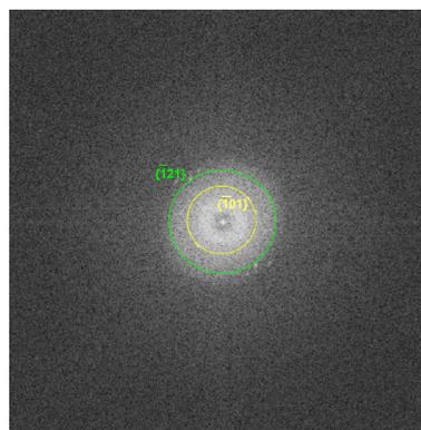
Figure 7. Indexed FFT pattern showing the  $\{\bar{1}01\}$  and  $\{\bar{1}21\}$  reflections.
