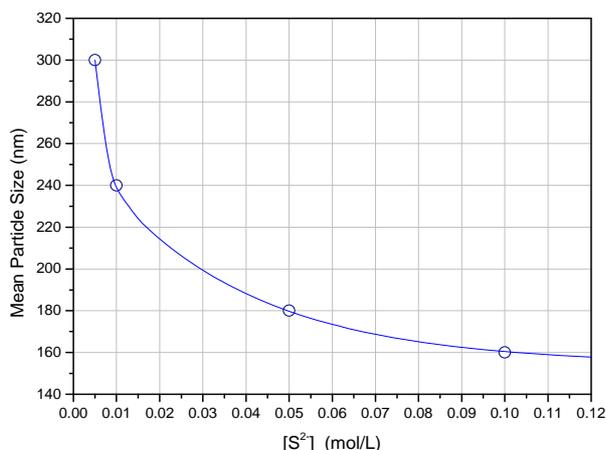
**Figure 1.** Average size of the Ag<sub>2</sub>S powders as a function of sulphide ions concentration obtained from dynamic light scattering measurements.
