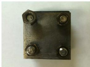
**Figure 1.** Press cell for making the sample in a pressed condition during the heat treatment.
