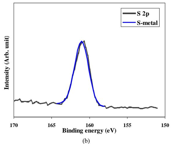
Figure 4. (a) XPS spectrum of S 2p energy level taken at the surface (a) and after 30 sec of Argon-ion sputtering (b) of the film annealed at 300°C.
