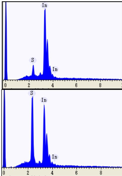
Figure 2. EDX measurement taken at one of the white particles distributed over the surface of the as-deposited (a) and 300°C-annealed (b) thin films.
