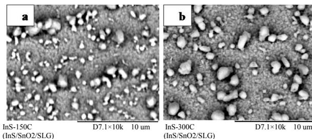
**Figure 1.** SEM measurements that show the surface morphology of films annealed at  $150^\circ\text{C}$  (a) and  $300^\circ\text{C}$  (b).
