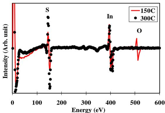
Figure 3. AES spectra of the films annealed at 150 and 300°C after 20 sec of Argon-ion sputtering.
