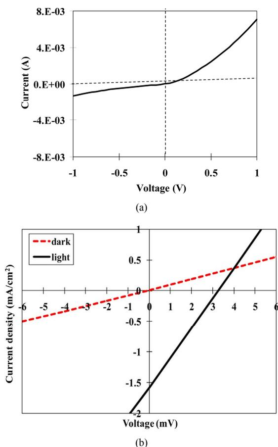
Figure 6. I-V characteristic of the [Glass/FTO/300°C-annealed  $\text{InS}_x\text{O}_y/\text{SnS}/\text{In}$ ] solar cells under dark (a) and illumination (b) conditions (solid line); dashed line is under dark.
