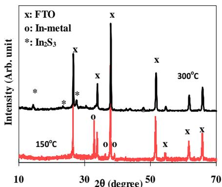
Figure 5. XRD spectra of films annealed at 150°C and 300°C.
