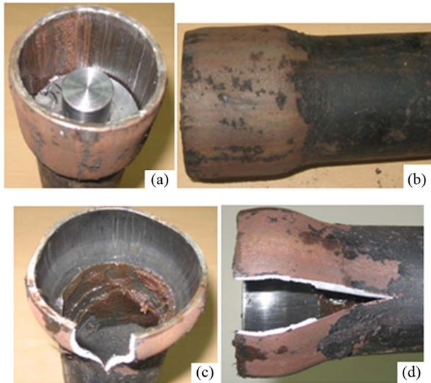
Figure 6. Expanded S40 pipes (a) and (b) uniform expansion at 15% expansion while (c) and (d) pipes cracked open at 25% expansion.
