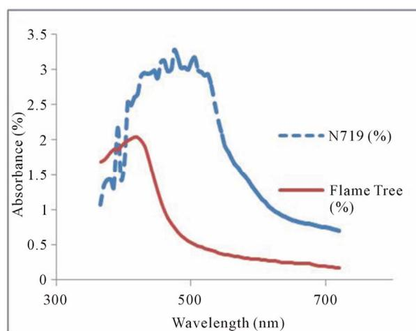
**Figure 3.** Absorption spectra of N719 dye and flame tree flower.
