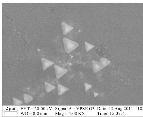
**Figure 2.** SEM image of fabricated TiO<sub>2</sub>.
