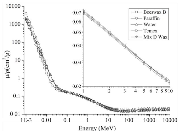
**Figure 4. Comparison of the behavior of the mass attenuation coefficients (obtained using the program Xcom) of beeswax B with other simulators.**
