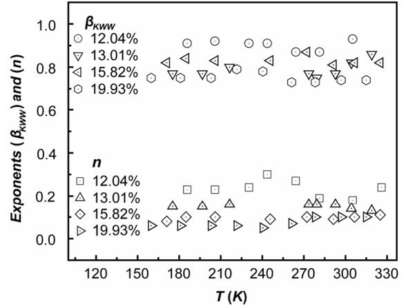
Figure 7. The temperature independence of the stretched exponent  $\beta_{KWW}$  obtained from fitting by KWW function and the exponent  $n$  from the conductivity power law.
