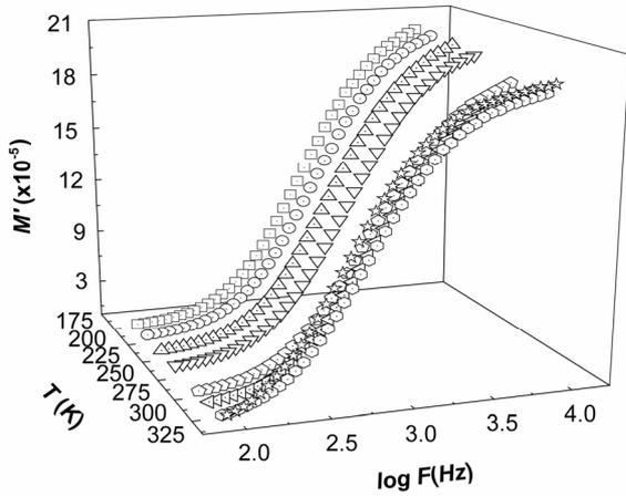
Figure 4. The variation of real part of the complex electric modulus,  $M'(\omega)$ , as a function of frequency and temperature, for 13.04%.
