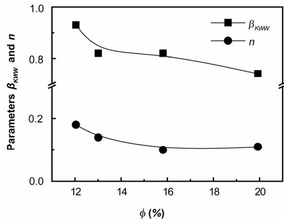
**Figure 3.** Electrical parameters,  $\beta_{KWW}$  (obtained from fitting by KWW function) and  $n$  (from the conductivity power law), as a function of volume concentrations of CB, at room temperature.
