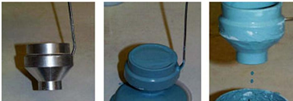
**Figure 8.** Measurement of viscosity with a flow cup [45].
