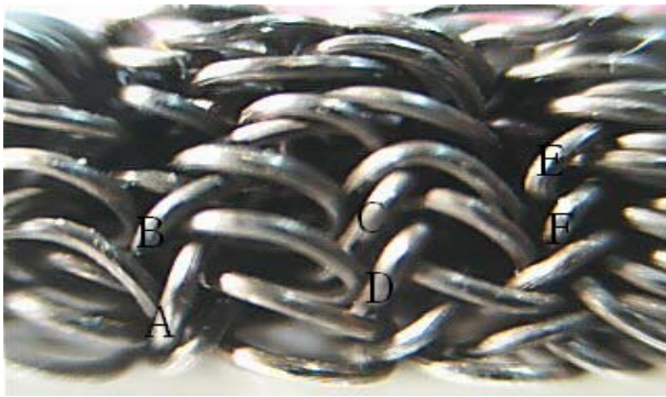
Figure 2. The mesoscopic feature of metallic wire on the side surface.
