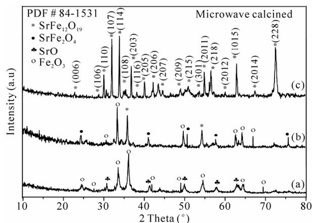
**Figure 4.** XRD patterns of the powders microwave calcined at different temperatures: (a) 500°C, (b) 750°C, and (c) 900°C for 10 minutes.
