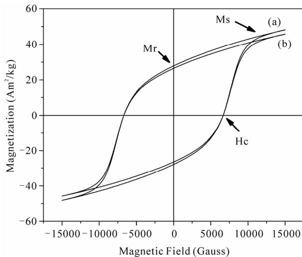
**Figure 7. Magnetization curve of SrFe<sub>12</sub>O<sub>19</sub> (a) powder conventionally calcined at 900°C for 3 h; (b) powder microwave calcined at 900°C for 10 minutes.**
