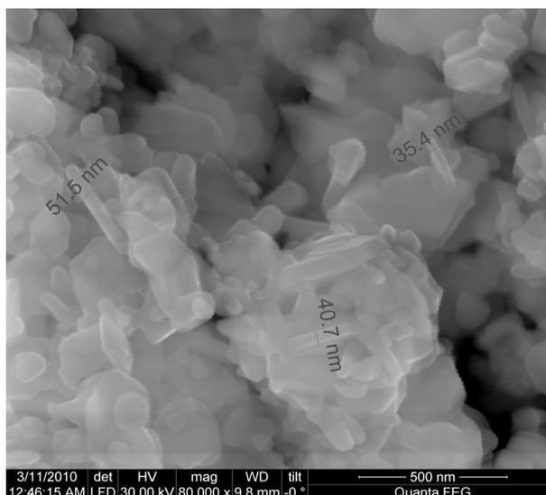
**Figure 6.** HR-SEM image of microwave calcined powder at 900°C for 10 minutes.
