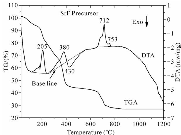
**Figure 1.** TG-DTA curves for the precursor.
