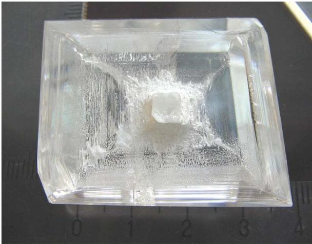
**Figure 1.** The as-grown KLuW crystal with seed orientations along  $b$  directions and severe cracks along  $a$  and  $(a + c)$  directions.
