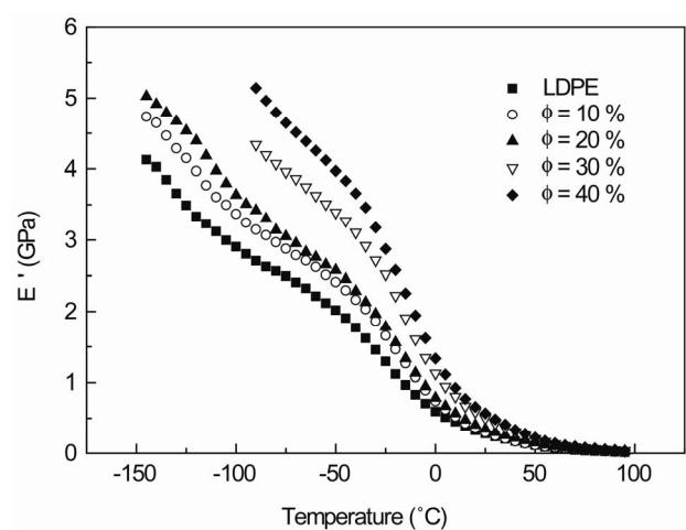
**Figure 1. Dependence of storage modulus on temperature of LDPE/GB5000 composite.**
