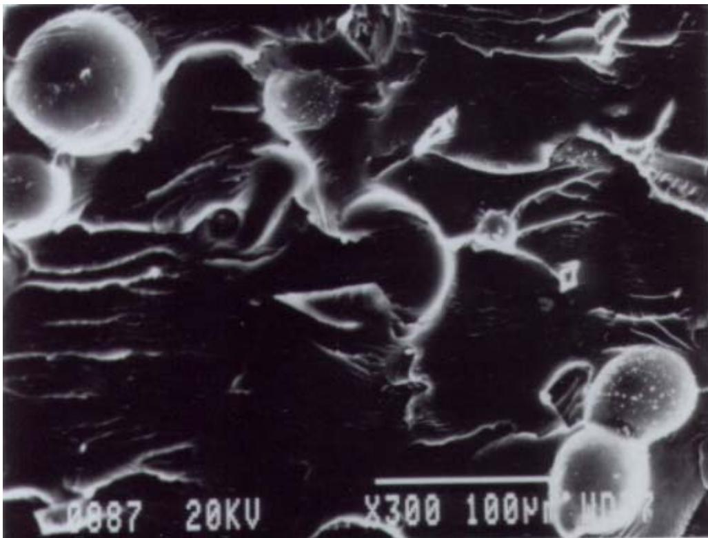
Figure 7. SEM photograph of fracture surface of LDPE/GB2429 composite.
