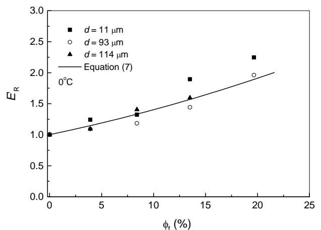
**Figure 5.** Relationship between relative storage modulus and GB volume fraction at  $0^\circ\text{C}$ .
