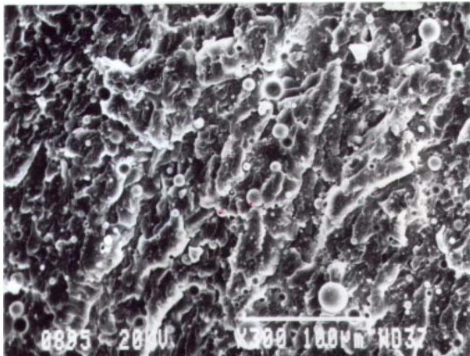
**Figure 8.** SEM photograph of fracture surface of LDPE/GB5000 composite.
