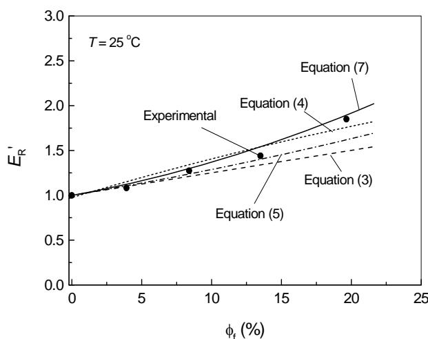
**Figure 9.** Comparison between predictions of relative storage moduli of LDPE/GB2429 system at 25°C.
