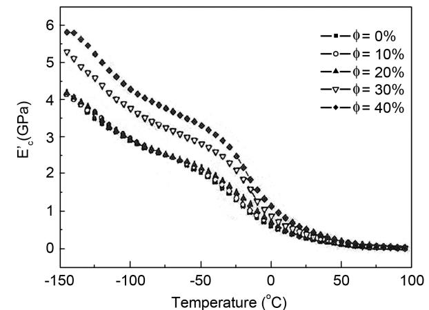
**Figure 2. Dependence of storage modulus on temperature of LDPE/GB2429 composite.**
