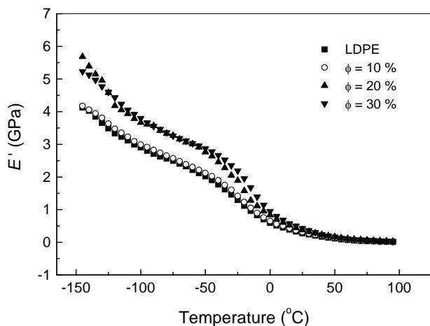
**Figure 3.** Dependence of storage modulus on temperature of LDPE/GB2227 composite.
