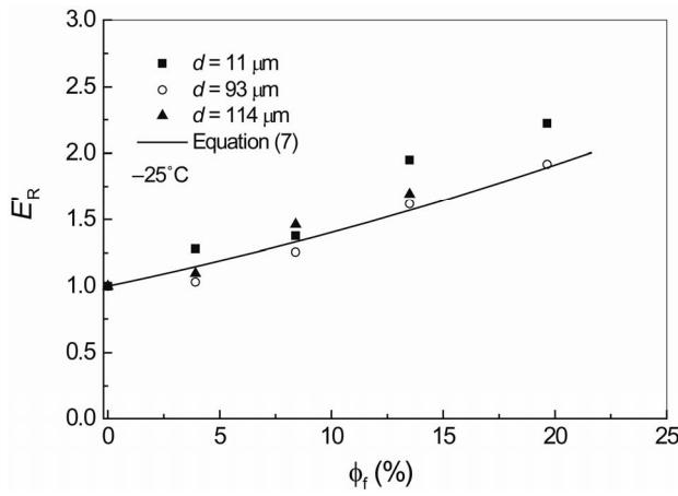
**Figure 4.** Relationship between relative storage modulus and GB volume fraction at  $-25^\circ\text{C}$ .
