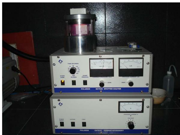
Figure 3. Evaporating metal coating (Au-Pd) in non-conductive samples.
