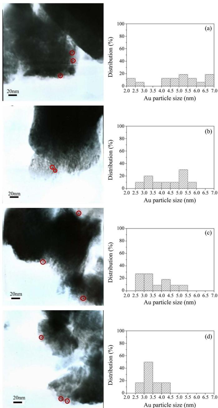
**Figure 2.** TEM images and Au particle diameter distributions of  $\text{Au}/\text{Mg}(\text{OH})_2\text{-CeO}_2$  catalysts with  $\text{Mg}/(\text{Mg} + \text{Ce})$  ratio = (a) 6.5%, (b) 20%, (c) 37.5%, (d) 50%.
