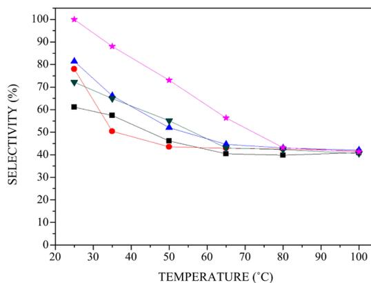
**Figure 8.** CO selectivity of Au/CeO<sub>2</sub> (■) and Au/Mg(OH)<sub>2</sub>-CeO<sub>2</sub> with different Mg/(Mg + Ce) ratios: 6.5% (●), 20% (▲), 37.5% (▼), 50% (★).
