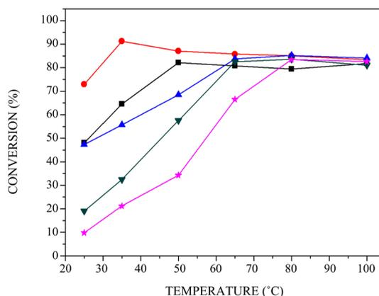
**Figure 7.** CO conversions of Au/CeO<sub>2</sub> (■) and Au/Mg(OH)<sub>2</sub>-CeO<sub>2</sub> with different Mg/(Mg + Ce) ratios: 6.5% (●), 20% (▲), 37.5% (▼), 50% (★).
