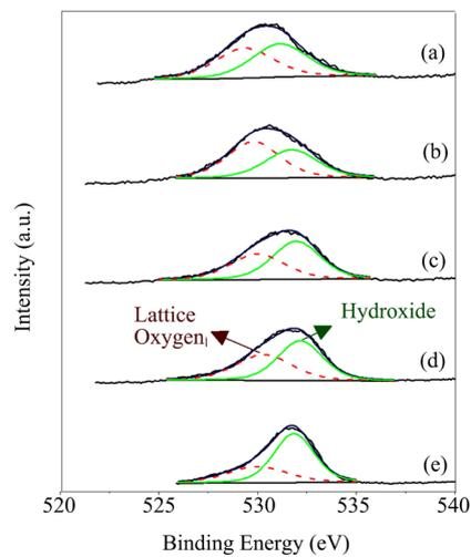
**Figure 5.** XPS O 1s spectra of Au/Mg(OH)<sub>2</sub>-CeO<sub>2</sub> catalysts with Mg/(Mg + Ce) = 6.5% (a), 20% (b), 37.5% (c), 50% (d), and Au/Mg(OH)<sub>2</sub> (e).
