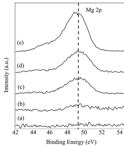
**Figure 4.** XPS Mg 2p spectra of Au/Mg(OH)<sub>2</sub>-CeO<sub>2</sub> catalysts with Mg/(Mg + Ce) = 6.5% (a), 20% (b), 37.5% (c), 50% (d), and Au/Mg(OH)<sub>2</sub> (e).
