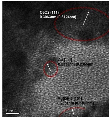
**Figure 3.** HR-TEM image of Au/Mg(OH)<sub>2</sub>-CeO<sub>2</sub> with Mg/(Mg + Ce) = 10%.
