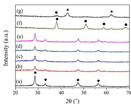
**Figure 1.** XRD pattern of Au/CeO<sub>2</sub> (a) and Au/Mg(OH)<sub>2</sub>-CeO<sub>2</sub> catalyst with Mg/(Mg + Ce) = 6.5% (b), 20% (c), 37.5% (d), 50% (e). Au/Mg(OH)<sub>2</sub> (f) and MgO support (g).
