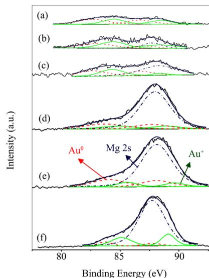
**Figure 6.** XPS Au 4f spectra of Au/CeO<sub>2</sub> (a), Au/Mg(OH)<sub>2</sub>-CeO<sub>2</sub> catalysts with Mg/(Mg + Ce) = 6.5% (b), 20% (c), 37.5% (d), 50% (e) and Au/Mg(OH)<sub>2</sub> (f).
