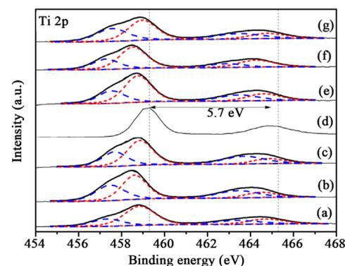
Figure 12. XPS Ti 2p spectra of the samples before reaction, (a) 1% CuO<sub>x</sub>-TiO<sub>2</sub>; (b) 3% CuO<sub>x</sub>-TiO<sub>2</sub>; (c) 5% CuO<sub>x</sub>-TiO<sub>2</sub>; (d) Au/TiO<sub>2</sub>; (e) Au/1%CuO<sub>x</sub>-TiO<sub>2</sub>; (f) Au/3%CuO<sub>x</sub>-TiO<sub>2</sub>; (g) Au/5%CuO<sub>x</sub>-TiO<sub>2</sub> (Ti<sup>3+</sup> is the dash line, and Ti<sup>4+</sup> is the short-dash line).
