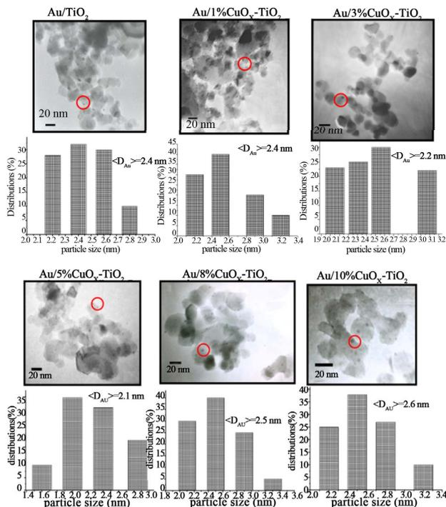
**Figure 2.** TEM images and particle size distributions of Au/CuO<sub>x</sub>-TiO<sub>2</sub> catalysts.
