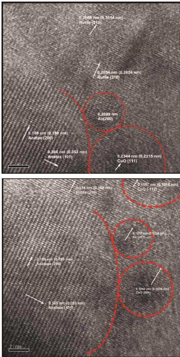
Figure 3. HRTEM image of Au/5% CuO<sub>x</sub>-TiO<sub>2</sub>.
