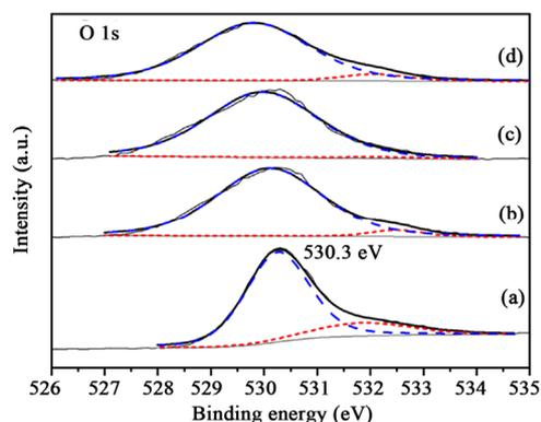
Figure 11. XPS O 1s spectra of the samples after reaction (a) Au/TiO<sub>2</sub>; (b) Au/1%CuO<sub>x</sub>-TiO<sub>2</sub>; (c) Au/3%CuO<sub>x</sub>-TiO<sub>2</sub>; (d) Au/5%CuO<sub>x</sub>-TiO<sub>2</sub> (O<sup>2-</sup> is the dash line, and OH<sup>-</sup> is the short-dash line).
