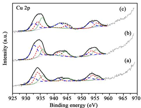
Figure 7. XPS Cu 2p spectra of (a) 1% CuO<sub>x</sub>-TiO<sub>2</sub> (c) 3% CuO<sub>x</sub>-TiO<sub>2</sub> (d) 5% CuO<sub>x</sub>-TiO<sub>2</sub> (Cu<sup>0</sup> is the dash line, and Cu<sup>+</sup> is the short-dash line).
