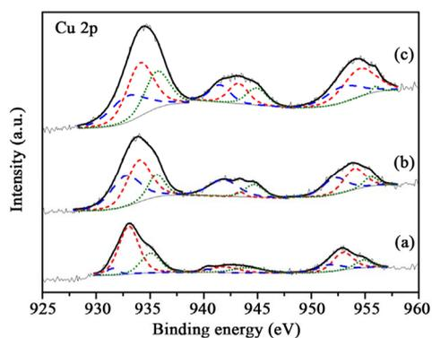
Figure 8. XPS Cu 2p spectra of the samples before reaction (a) Au/1%CuO<sub>x</sub>-TiO<sub>2</sub>; (c) Au/3%CuO<sub>x</sub>-TiO<sub>2</sub>; (d) Au/5% CuO<sub>x</sub>-TiO<sub>2</sub> (Cu<sup>0</sup> is the dash line, and Cu<sup>+</sup> is the short-dash line).
