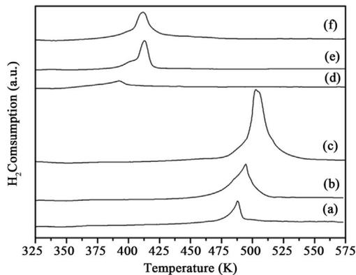
Figure 4. TPR profiles of the catalysts, (a) 1% CuO<sub>x</sub>-TiO<sub>2</sub>; (b) 3% CuO<sub>x</sub>-TiO<sub>2</sub>; (c) 5% CuO<sub>x</sub>-TiO<sub>2</sub>; (d) Au/1%CuO<sub>x</sub>-TiO<sub>2</sub>; (e) Au/3%CuO<sub>x</sub>-TiO<sub>2</sub>; (f) Au/5%CuO<sub>x</sub>-TiO<sub>2</sub>.
