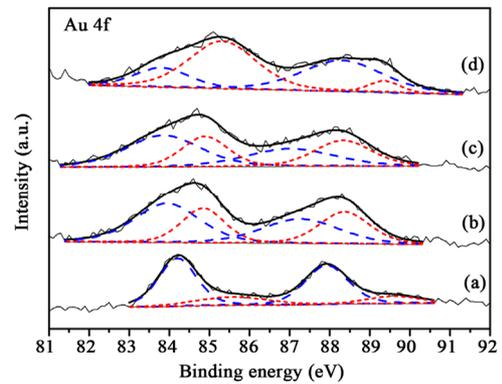
Figure 5. XPS Au 4f spectra of (a) Au/TiO<sub>2</sub> (b) Au/1% CuO<sub>x</sub>-TiO<sub>2</sub> (c) Au/3%CuO<sub>x</sub>-TiO<sub>2</sub> (d) Au/5%CuO<sub>x</sub>-TiO<sub>2</sub> before reaction. Au<sup>0</sup> is the dash line, and Au<sup>+</sup> is the short-dash line).
