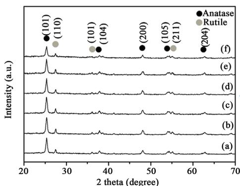
**Figure 1.** XRD of patterns of Au/CuO<sub>x</sub>-TiO<sub>2</sub>, (a) Au/TiO<sub>2</sub>; (b) Au/1%CuO<sub>x</sub>-TiO<sub>2</sub>; (c) Au/3%CuO<sub>x</sub>-TiO<sub>2</sub>; (d) Au/5%CuO<sub>x</sub>-TiO<sub>2</sub>; (e) Au/8%CuO-TiO<sub>2</sub>; (f) Au/10%CuO<sub>x</sub>-TiO<sub>2</sub>.
