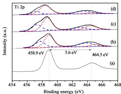
**Figure 13. XPS Ti 2p spectra of the samples after reaction, (a) Au/TiO<sub>2</sub>; (b) Au/1%CuO<sub>x</sub>-TiO<sub>2</sub>; (c) Au/3%CuO<sub>x</sub>-TiO<sub>2</sub>; (d) Au/5%CuO<sub>x</sub>-TiO<sub>2</sub> (Ti<sup>3+</sup> is blue dash line, and Ti<sup>4+</sup> is red dash line).**
