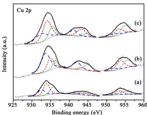
Figure 9. XPS Cu 2p spectra of the samples after reaction (a) Au/1%CuO<sub>x</sub>-TiO<sub>2</sub>; (c) Au/3%CuO<sub>x</sub>-TiO<sub>2</sub>; (d) Au/5% CuO<sub>x</sub>-TiO<sub>2</sub> (Cu<sup>0</sup> is the dash line, and Cu<sup>+</sup> is the short-dash line).
