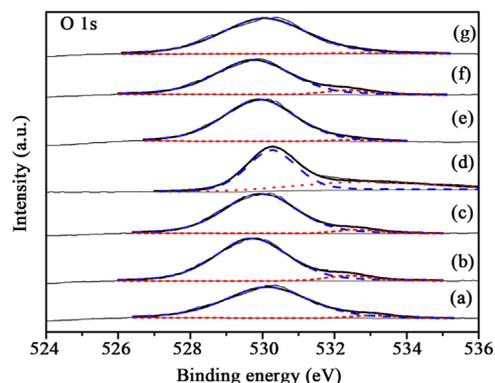
Figure 10. XPS O 1s spectra of the samples before reaction (a) 1% CuO<sub>x</sub>-TiO<sub>2</sub>; (b) 3% CuO<sub>x</sub>-TiO<sub>2</sub>; (c) 5% CuO<sub>x</sub>-TiO<sub>2</sub>; (d) Au/TiO<sub>2</sub>; (e) Au/1%CuO<sub>x</sub>-TiO<sub>2</sub>; (f) Au/3%CuO<sub>x</sub>-TiO<sub>2</sub>; (g) Au/5%CuO<sub>x</sub>-TiO<sub>2</sub> (O<sup>2-</sup> is the dash line, and OH<sup>-</sup> is the short-dash line).
