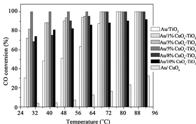
**Figure 14.** The CO conversion on Au/CuO<sub>x</sub>-TiO<sub>2</sub> catalysts. (Reactant gas: 1% CO in air;  $WHSV=120,000$  ml/h·g).
