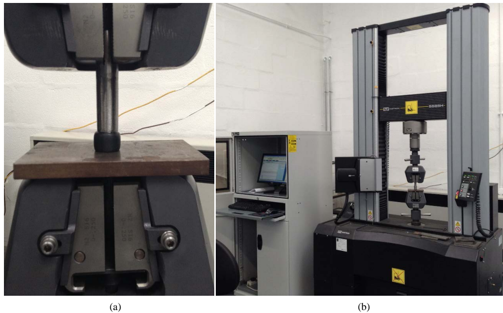
Figure 6. Experimental setup for compression test (a) test machine (b) compressed specimen.
