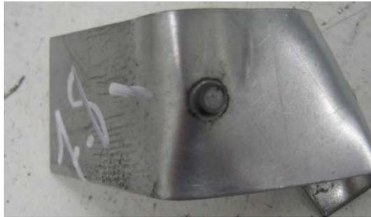
Figure 3. Coach-peel tested coupon.
