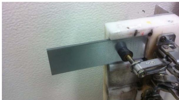
**Figure 2.** Welding fixture before welding.
