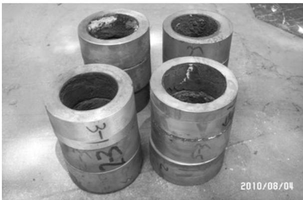
**Figure 5.** The picture of high speed steel roll after machining outer surface.
