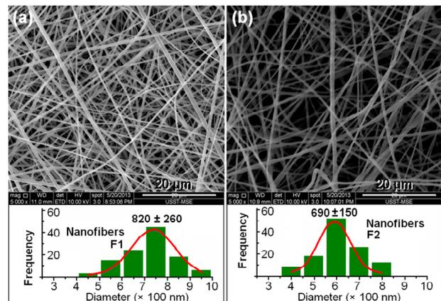
**Figure 4.** FESEM images of the nanofibers from different spinneret and their diameters' distributions: (a) an EP-coated spinneret, (b) a traditional stainless steel capillary.
