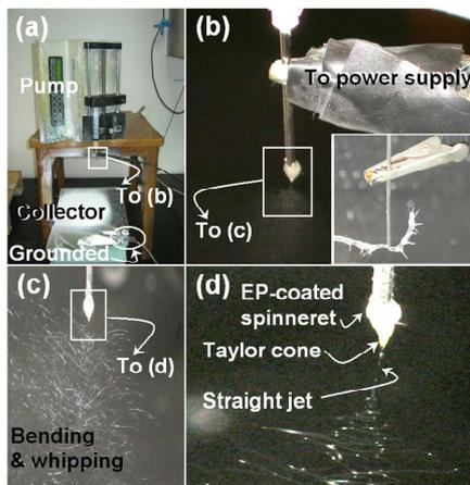
**Figure 2.** The arrangement of the apparatus (a and b) and observations of the electrospinning process (c and d). The inset in b shows a typical clogging in an electrospinning process using a metal spinneret.
