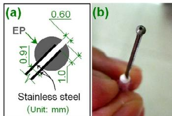
**Figure 1.** The design of an epoxy-coated spinneret head (a) and its digital photo (b).
