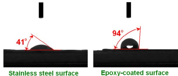
**Figure 3.** Experiments to investigate the influence of spinneret composition on the electrospinning process, the contact angle of a spinnable solution on a stainless steel plate and on an EP-coated plate.
