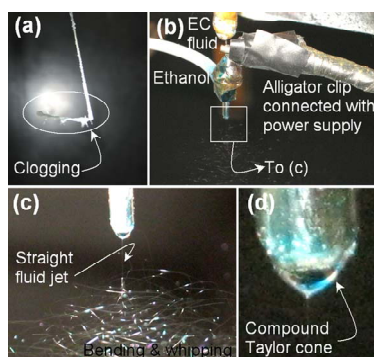
Figure 2. Observations of the modified coaxial electrospinning and a single fluid process: (a) a typical clogging of the single fluid electrospinning; (b) a digital picture shows the connection of the concentric spinneret with the syringe pump and the power supply; (c) a typical coaxial electrospinning process with ethanol as sheath fluid and under a sheath-to-core flow rate ratio of 0.25 (taken under a magnification of 12 \times ); (d) the compound Taylor cone.
