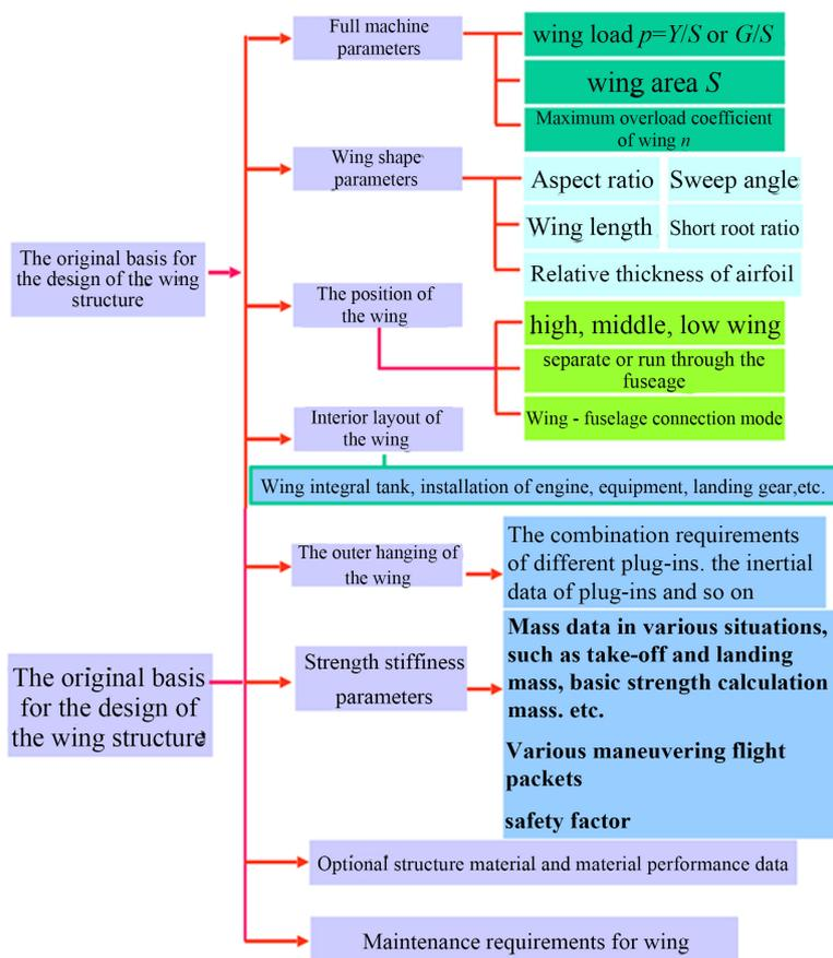
Figure 4. The original basis of wing design.
