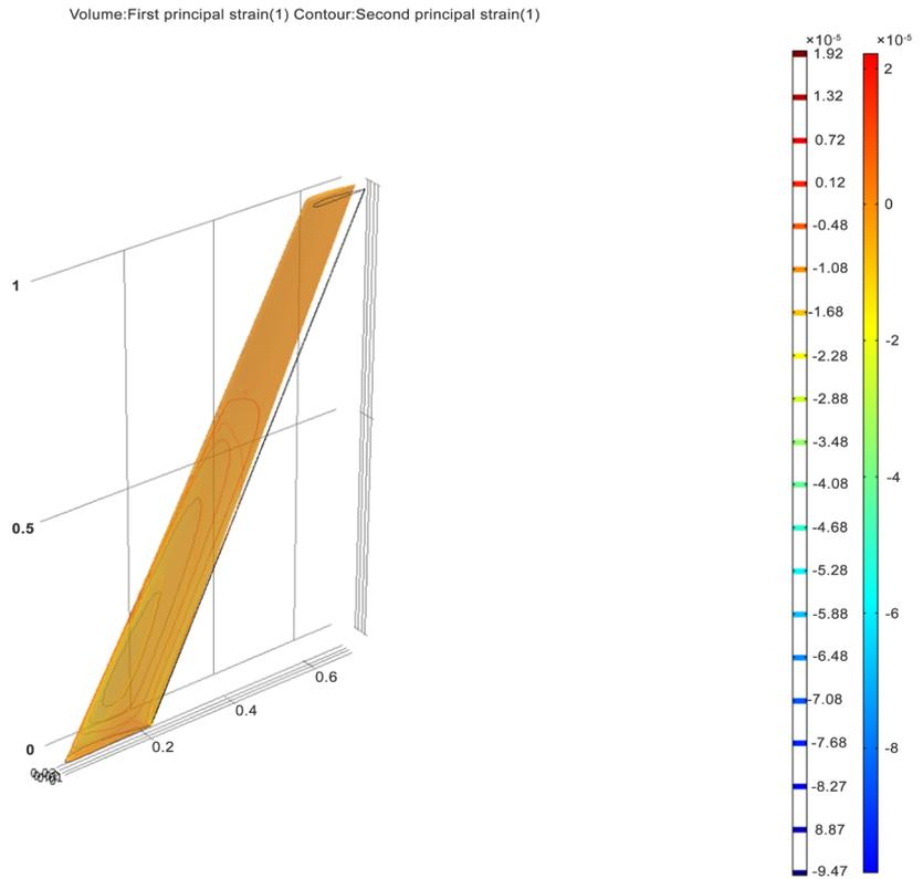
Figure 9. Second principle strain cloud map.
