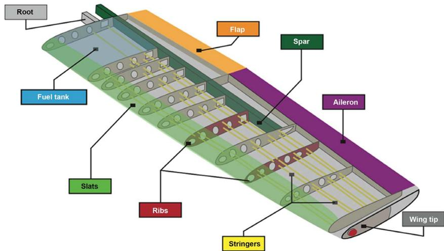
**Figure 3.** Structure of a straight beam wing [4].
