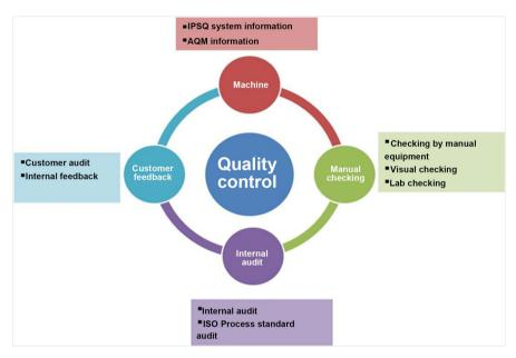
Figure 3. Quality control methods in the painting process.
