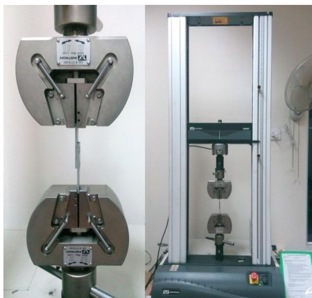
Figure 4. Tensile shear test machine along the entire weld length.
