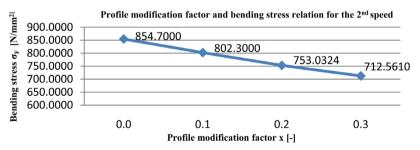
Figure 21. Profile modification factor and bending stress relation for the 2<sup>nd</sup> speed.
