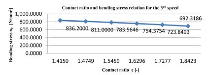
Figure 10. Contact ratio and bending stress relation for the 3<sup>rd</sup> speed.
