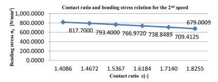
Figure 9. Contact ratio and bending stress relation for the 2<sup>nd</sup> speed.
