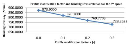
Figure 22. Profile modification factor and bending stress relation for the 3rd speed.
