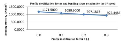
Figure 20. Profile modification factor and bending stress relation for the 1st speed.
