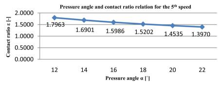
Figure 18. Contact ratio and pressure angle relation for the 5<sup>th</sup> speed.
