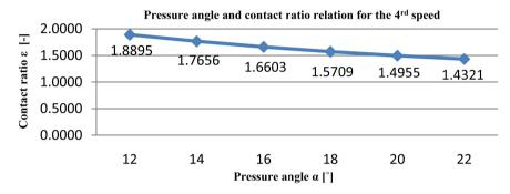
Figure 17. Contact ratio and pressure angle relation for the 4<sup>th</sup> speed.
