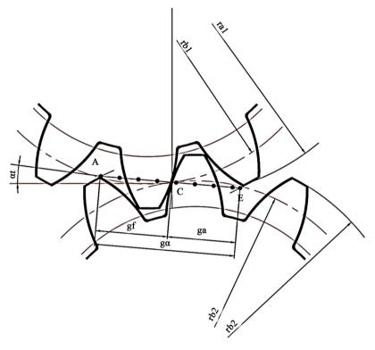
Figure 4. Contac line of helical gear including contact length AE.
