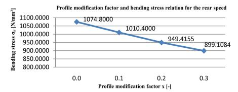
Figure 25. Profile modification factor and bending stress relation for the rear speed.
