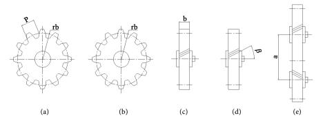
Figure 2. Design parameters for a gearbox. (a) module; (b) number of teeth z; (c) facewidth b; (d) helix angle  $\beta$ ; (e) centre distance a.
