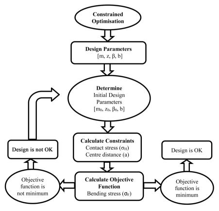
Figure 7. Flow chart to optimise gearbox design parameters.
