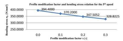
Figure 24. Profile modification factor and bending stress relation for the 5th speed.
