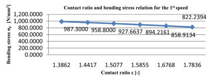
Figure 8. Contact ratio and bending stress relation for the 1st speed.
