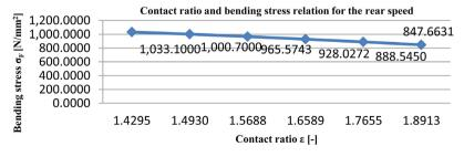
Figure 13. Contact ratio and bending stress relation for the rear speed.
