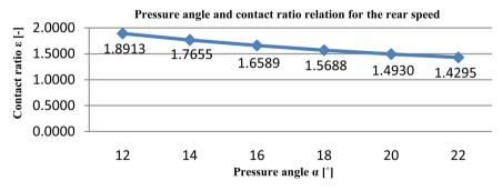
Figure 19. Contact ratio and pressure angle relation for the rear speed.
