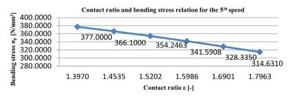
Figure 12. Contact ratio and bending stress relation for the 5<sup>th</sup> speed.
