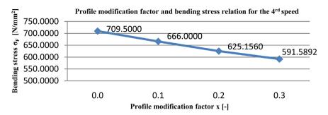
**Figure 23.** Profile modification factor and bending stress relation for the 4<sup>th</sup> speed.
