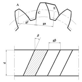
Figure 3. Contac line of helical gear.
