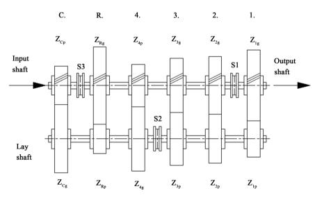
Figure 1. Five-Speed manual gearbox with helical gear for automotive transmission.
