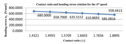
Figure 11. Contact ratio and bending stress relation for the 4<sup>th</sup> speed.
