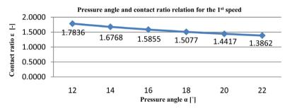
Figure 14. Contact ratio and pressure angle relation for the 1st speed.
