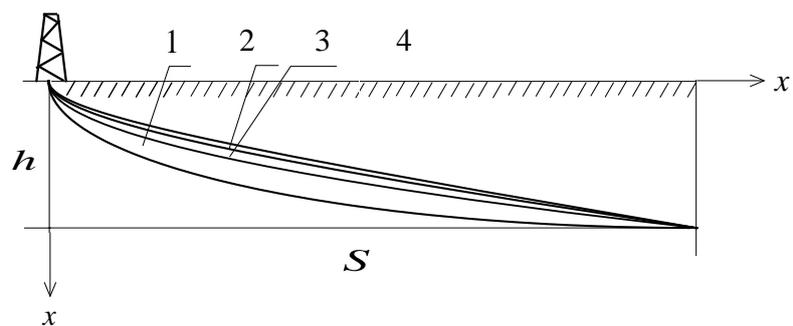
**Figure 1.** Geometrical layout of wells of the elliptical (1), parabolic (2) and hyperbolic (3,  $e = 1.01$ ; 4,  $e = 1.015$ ) shapes ( $h = 1000m, S = 4000m$ ) {where the ellipse equation is  $S^2/a^2 + h^2/b^2 = 1$ , parabola:  $4pS = h^2$ , hyperbola:  $S^2/a^2 - h^2/b^2 = 1$ ,  $a, b$ , and  $p$  are constants}.
