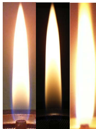
Figure 2. Flames visible height of 50 mm, considering the fuels CH 4 , NGV and LPG, from left to right.
