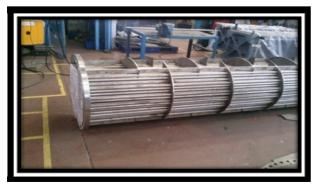
Figure 5. Tubes & Baffles assembly.
