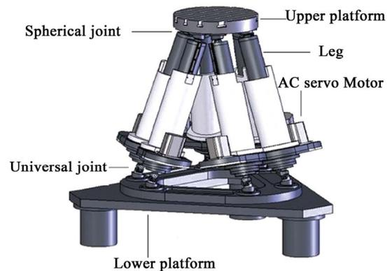
**Figure 2.** Typical Gough Stewart platform [9].
