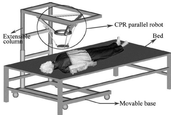
**Figure 18. Conceptual design of Cardio-pulmonary resuscitation (CPR) operation [27].**
