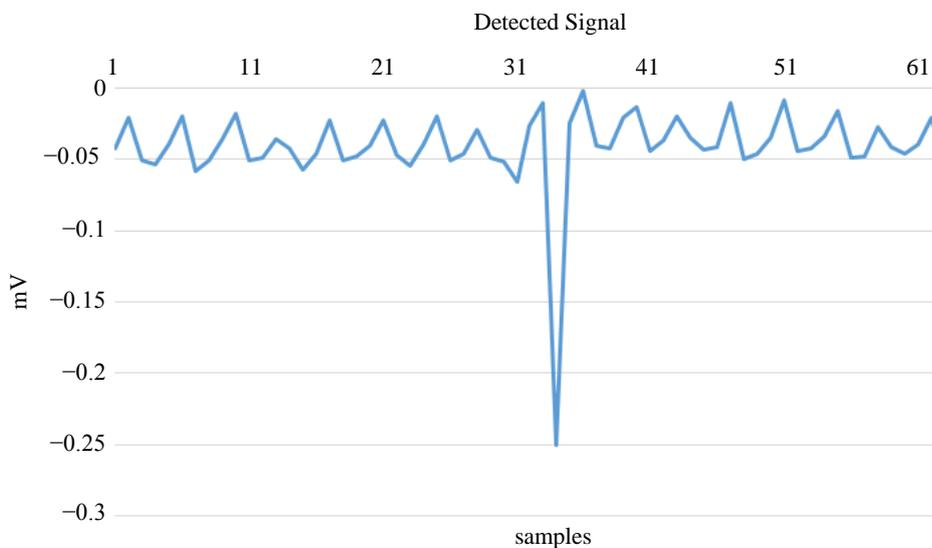
**Figure 8.** Detected resonant signal from a suspension of  $\text{CH}_3\text{OH}$  and  $\text{H}_2\text{O}$  with a 100 MHz source signal in a  $1.48 \text{ T} \pm 0.1 \text{ T}$  magnetic field, as recorded with the DAQ in time-domain.
