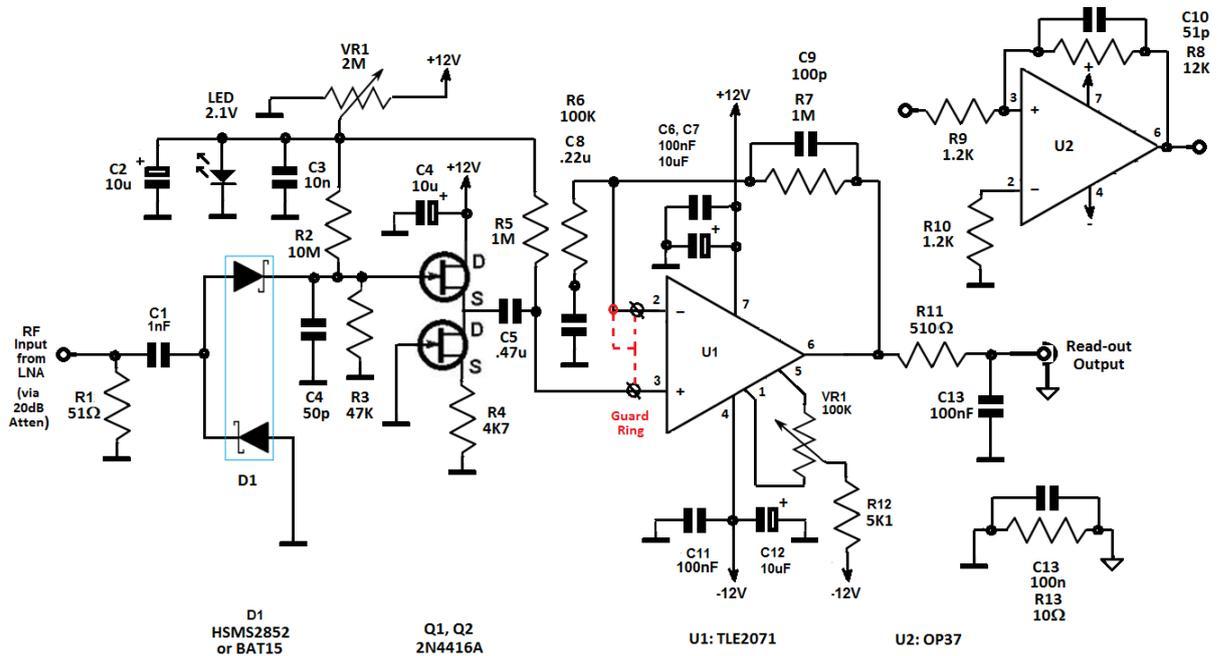
**Figure 3.** A block schematic of the zero-bias Schottky Barrier Diode (SBD) detection system following the LNA stage, based upon HSMS-2850 ZBD's and a precision low-noise RF post-amplifier built around a precision TLE2071 low noise high-speed jFET operational amplifier. An optional ~250 KHz Low-Pass Filter (LPF), based on OP37/OP27 shown in the inset, can be added to output for optimal signal processing.
