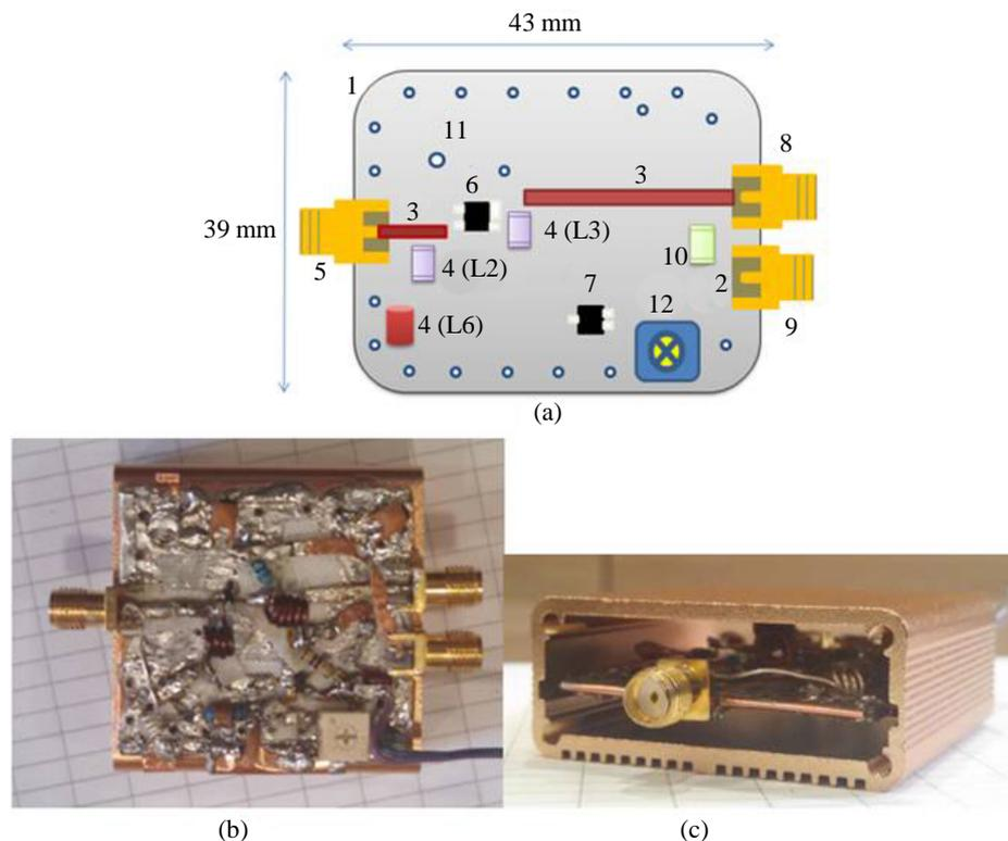
**Figure 4.** a) The suggested layout for the ULNA board. 1. FR4/PTFE Board, 2. Teflon Strip, 3. 50 Ω Micro-strip, 4. Inductors (this prototype used hand-wound inductors which were later replaced in following prototypes with HiQ SMD inductors), 5. SMA Connector, 6. HEMT transistor, 7. BJT transistor, 8. RF OUT, 9. DC OUT, 10. F/T LC Filter, 11. Via Holes, 12. Potentiometer, b) A photograph of our prototype; c) Cross sectional view of the unit while mounted in the case.
