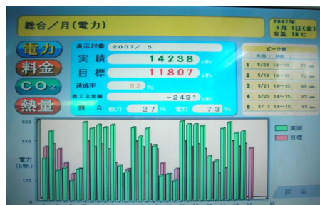
Figure 2. Energy-saving navigator. Power consumption data are sent from the power distribution board (top left) to the energy-saving navigator, and displayed on the monitor (top right). An example of the monitor display (bottom).
