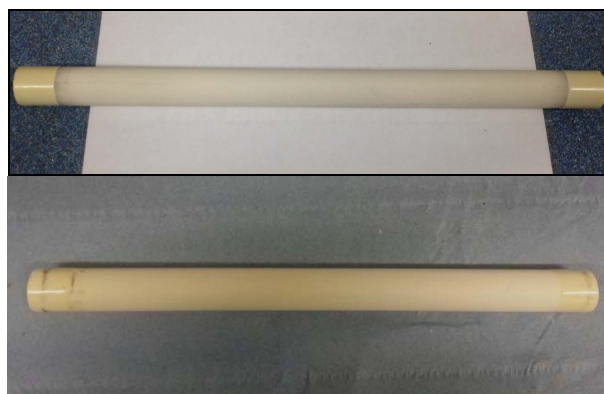
Figure 1. Tubular ceramic support (top) and nano-structured composite (bottom).
