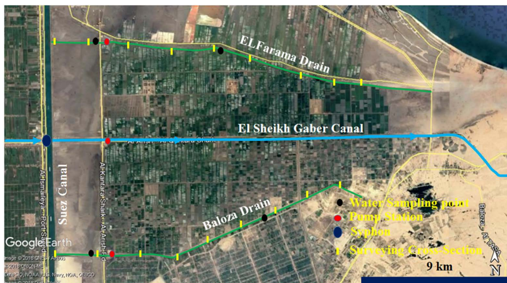
Figure 2. Hydrographic survey cross-sections locations and water sample locations.
