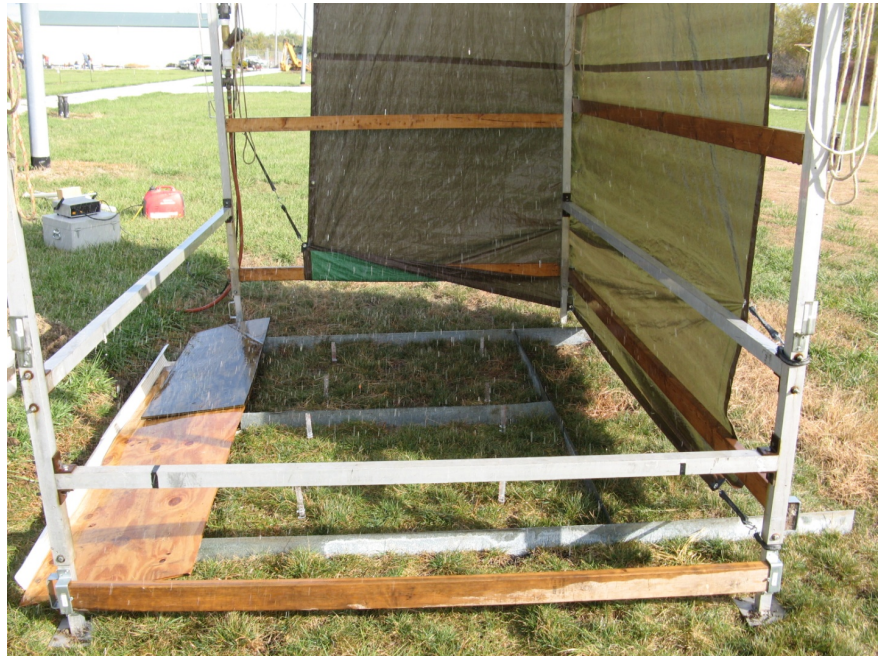
Figure 3. Rainfall simulation on side-by-side small plots in 2012. Note the tarp was used to block the wind and increase uniformity of simulated rainfall on the plots. Four small rain gages in each plot were used to assess the rainfall distribution.
