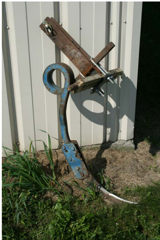
Figure 1. Homemade soil slotting tool used in Experiment 1.
