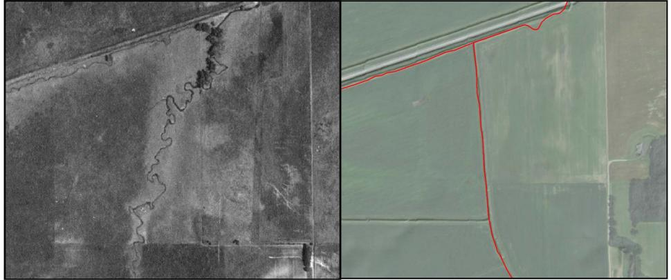
**Figure 3.** Aerial imagery from 1938 (left) and 2013 NAIP imagery (right) in bass creek watershed. Notice the change in direction the watercourse takes after ditching indicating alterations.
