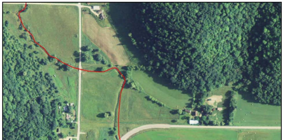
**Figure 2.** Altered stream reach in west fork Knapp creek watershed. Note surrounding agricultural land and roads disrupting natural flow and decreasing sinuosity.
