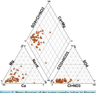
Figure 5. Piper diagram of the water samples taken in November 2012.
