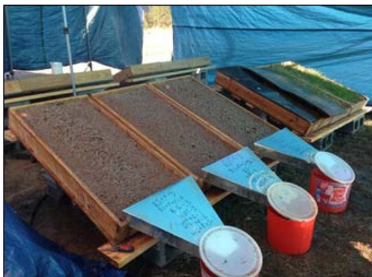
Figure 2. Collection of runoff from test plots, TGRU, Auburn, AL.
