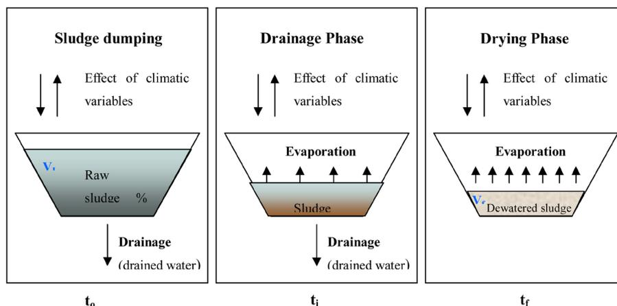
**Figure 2.** Schematic illustration of the Drainage Bed dewatering and variables involved.
