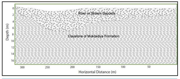
Figure 3. Geologic cross section for the proposed subsurface dam's selected site location.
