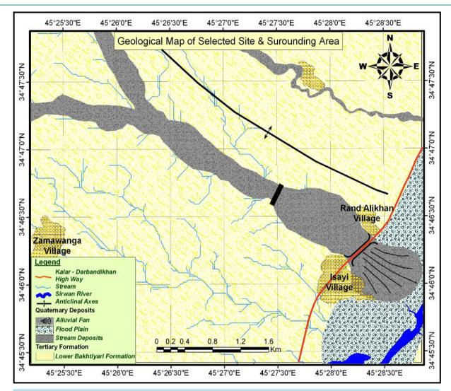
Figure 2. Geological map of the selected site location for construction of subsurface dam.
