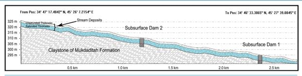
Figure 11. Longitudinal section along Isayi stream, illustrating location of the suggested subsurface dams with the stream deposits.
