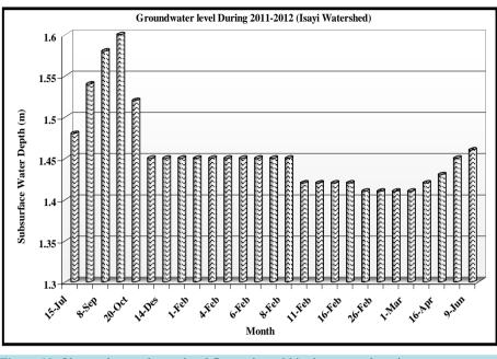
Figure 10. Observed groundwater level fluctuation within the stream deposits.
