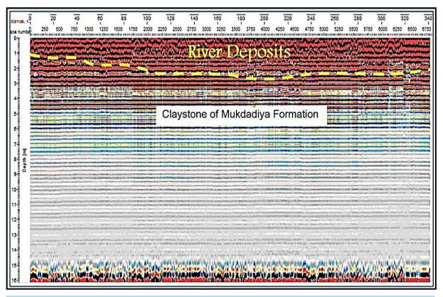
Figure 5. Radar section of the profile NO.2.
