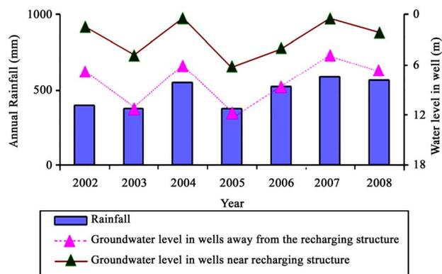
Figure 2. Effects of groundwater recharging structures on mean groundwater level in open wells, Gokulpura-Goverdhanpura watershed, Bundi, Rajasthan India, 2002-2008.
