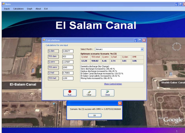
Figure 6. Screen displaying the original and calculated control actions at the feeding points along El-Salam Canal for January 2007.
