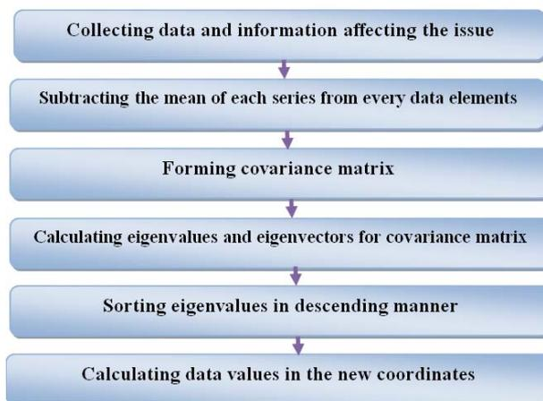
Figure 2. Steps of Principle Component Analysis.
