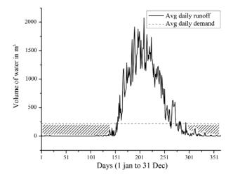
Figure 3. Mass balance representation of storage volume.
