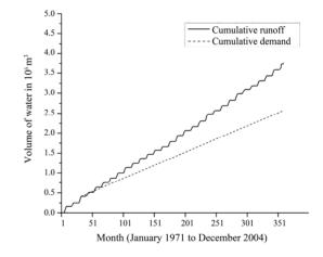
Figure 4. Ripple diagram method adopted.
