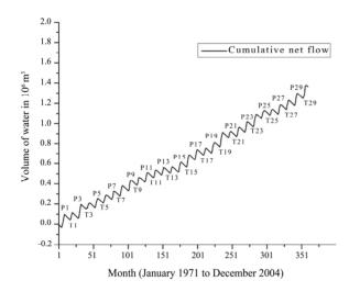
Figure 5. Results of Sequent peak algorithm method.
