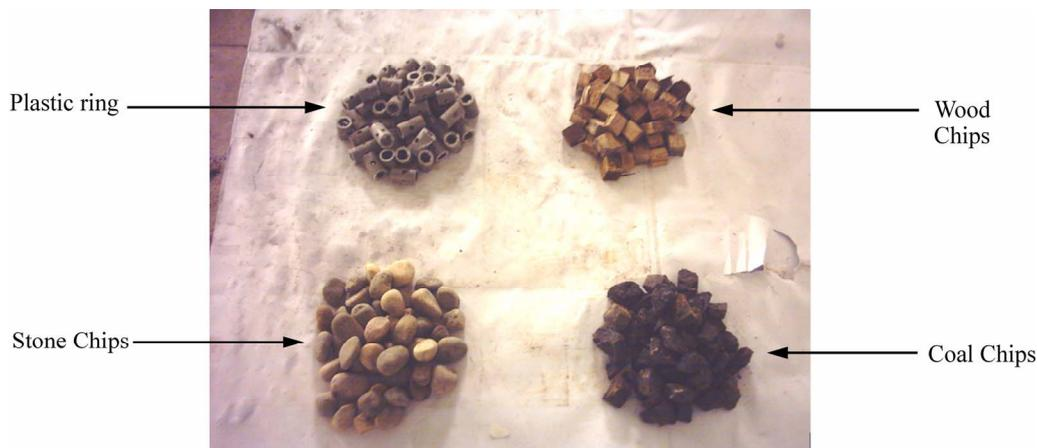
Figure 2. Different types of materials used as packing materials.
